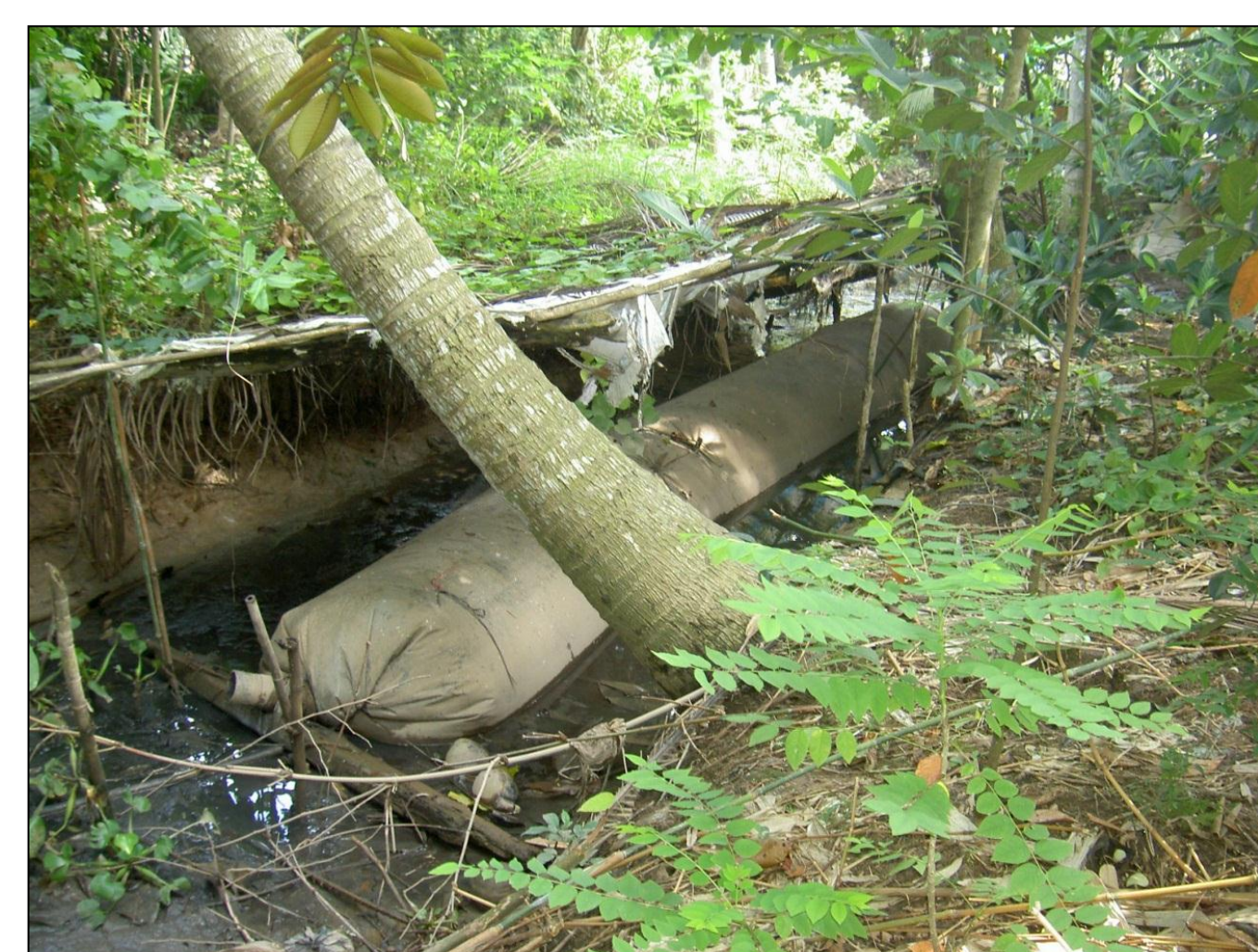
Plastic biogas plant for the treatment of animal waste
